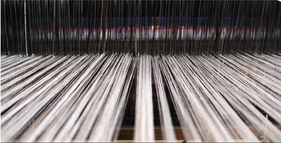
Warp yarns longitudinally arranged in the loom
