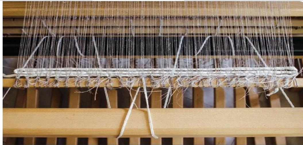
Warp yarns longitudinally arranged in the loom
