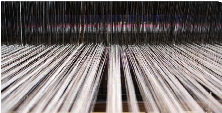
Warp yarns longitudinally arranged in the loom
