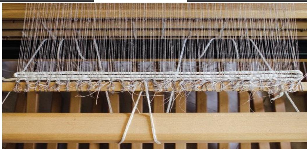
Warp yarns longitudinally arranged in the loom
