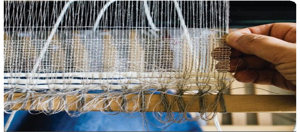
Warp yarns longitudinally arranged in the loom and fabric
