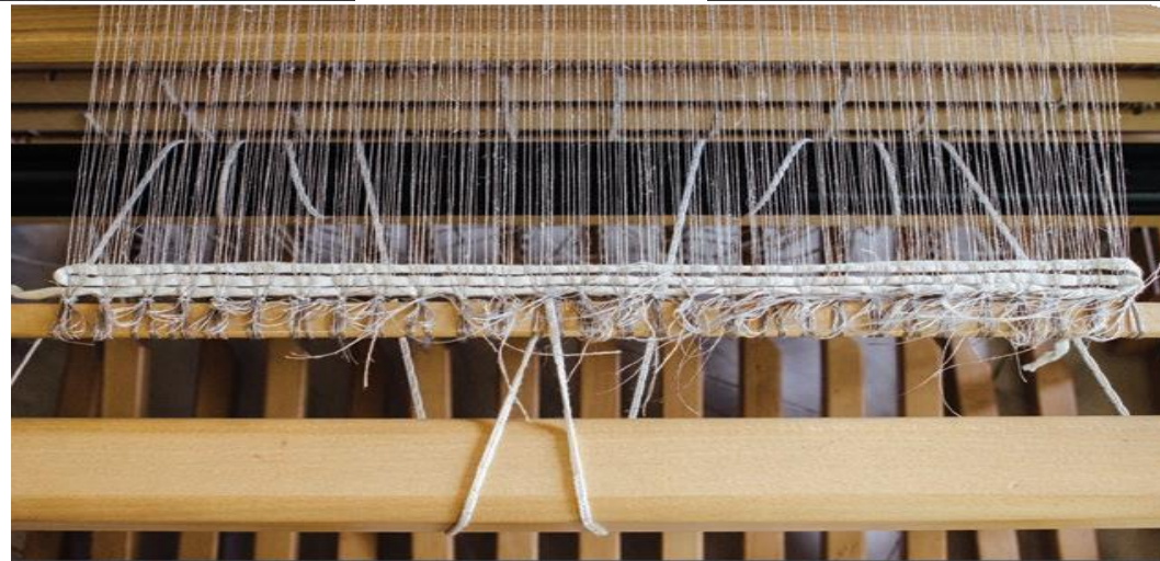
Warp yarns longitudinally arranged in the loom
