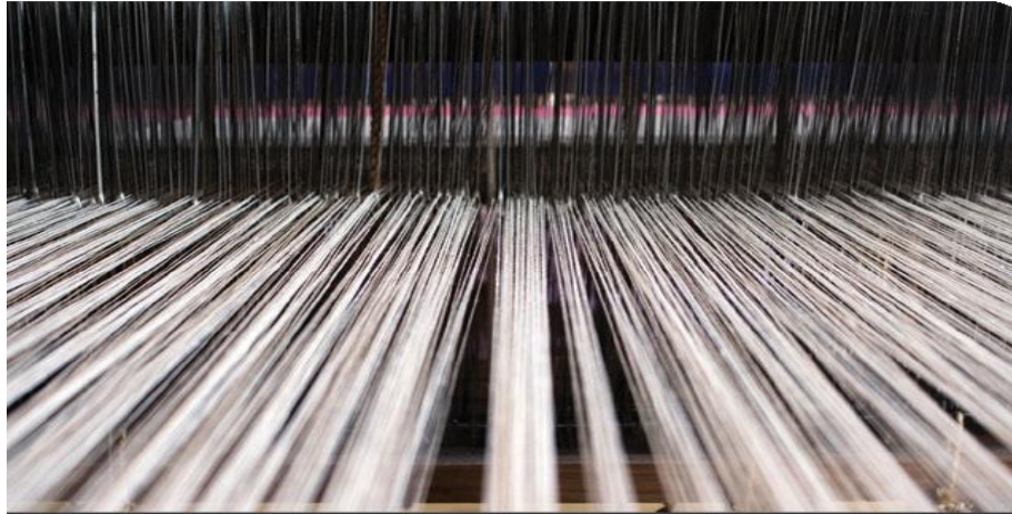
Warp yarns longitudinally arranged in the loom
