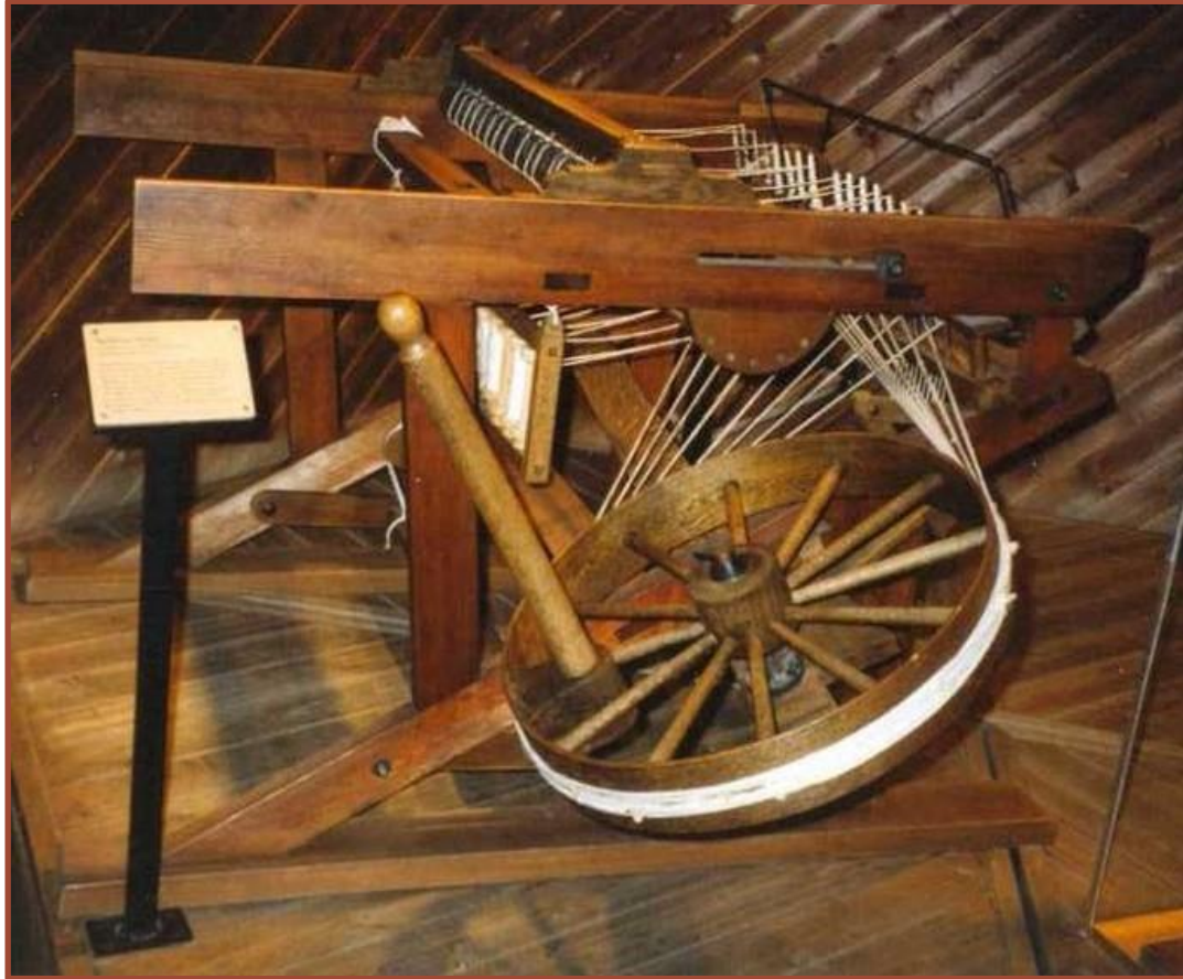
The spinning wheel (spinning Jenny) invented by James Hargreaves, 1765.
