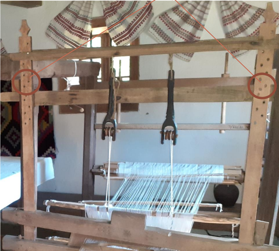
f. Upright posts
