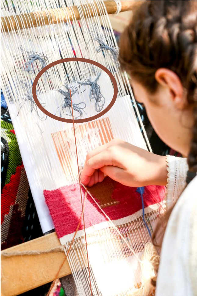
The shed is picked by a heddle made by strings
