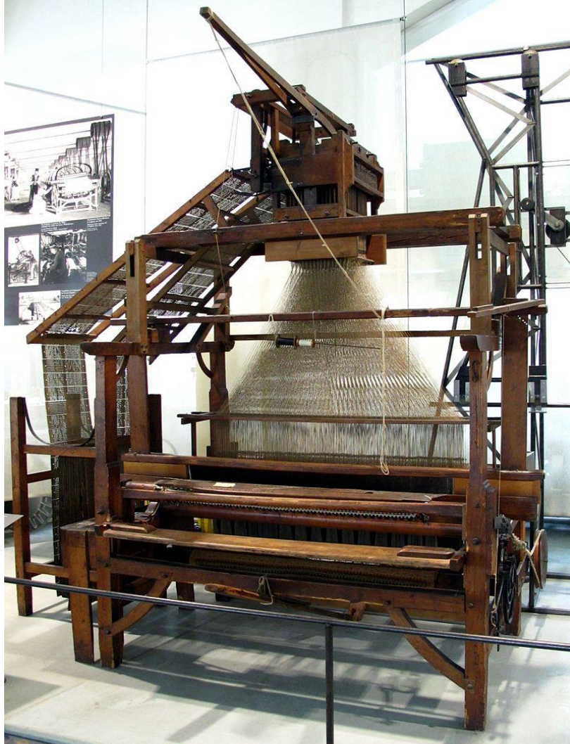
Carpet loom with Jacquard apparatus by Carl Engel, Nördlingen, around 1860.
