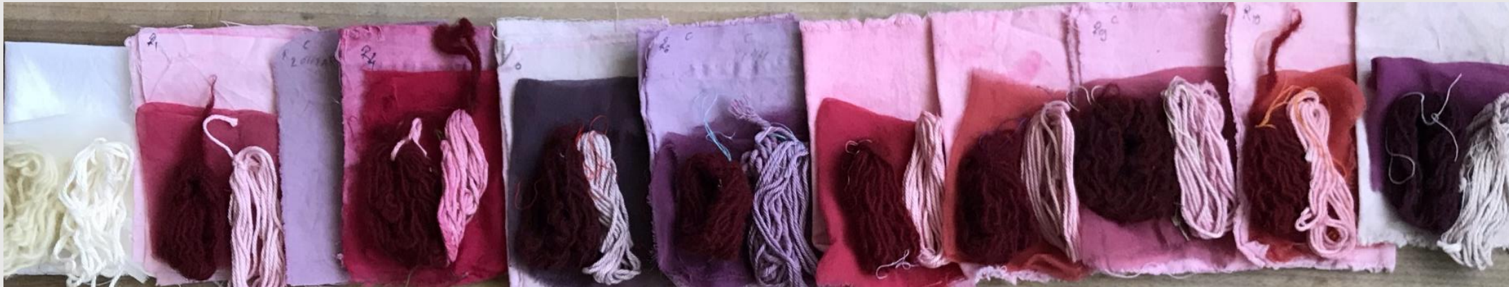
No color, No mordant, sumac alum Iron Copper Tin Vinegar Salt Citric Acid Wood ash
