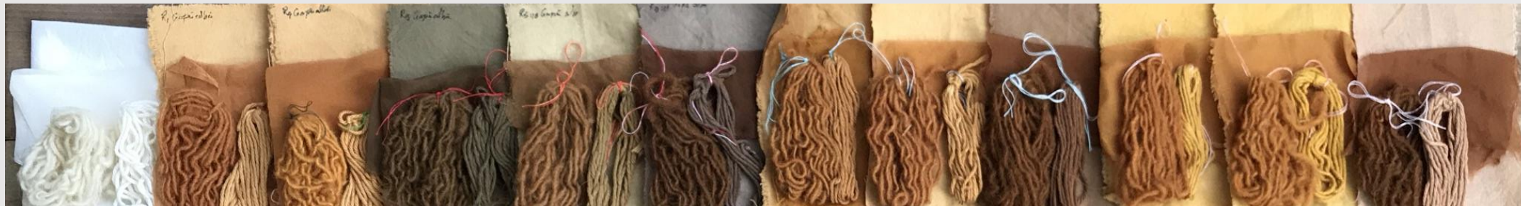
No color, No mordant, alum Iron iron+ citric iron wood ash Copper Copper citric Copper wood ash Tin Tin citric tin wood ash
