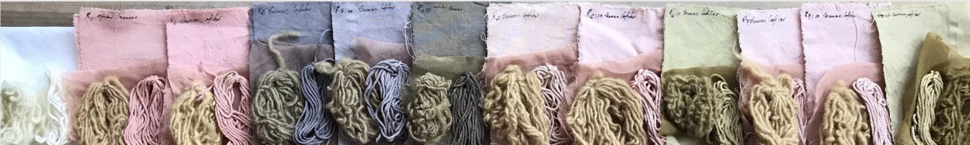
No color, No mordant, alum Iron iron+ citric iron wood ash Copper Copper citric Copper wood ash Tin Tin citric tin wood ash
